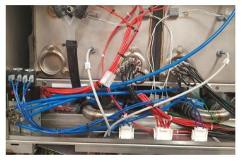
Locate and mount the below shown multi plugs in the top plate - behind the electrical panel.
