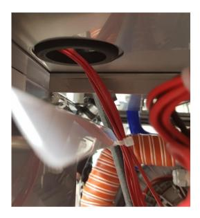
The bundle contains following wires: 20-6 / 3L2 for V1, 20-7 / 3L2 for V2, 20-8 / 3L2 for V3 (Option), 20-13 / 3L2 for V4 (Tank 1), 21-4 / 3L2 for V5 (Tank 2) and 21-1 / 3L2 for V6 (cooling drain) -connect them to matching numbered wires in the connection plinths shown below:
