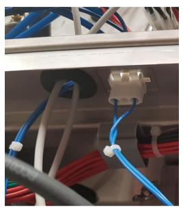
Wire 13-13 / 13-14 must be connected to the level sensor of tank 2 (left) and wire 13-15 / 13-16 must be connected to the level sensor of tank 1 (right):
