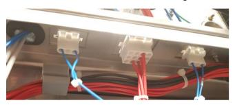
Connect the plug of the left pneumatic valve to the left plug and the plug of the right pneumatic valve to the right plug. Connect the 12-pole plug with red wires to the matching plug in the front. Thermo sensor B32 must be mounted in tank 2 (left) and B51 in tank 1 (right).
