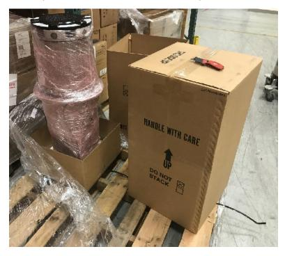
iv. Invert the emitter onto a flattened box or included foam.
