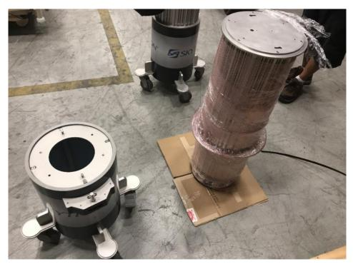
v. Place the inverted base atop the inverted emitter, ensuring the shoulder bolts slide into emitter's bottom plate. The base with the pull pin goes with the even numbered unit and the base with the slot goes with the odd numbered, primary emitter.
