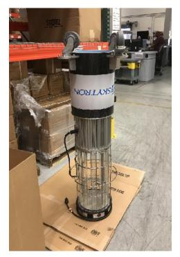
vi. Rotate the base clockwise to lock into position. When locked into position, thread and tighten two fasteners, included in accessories, into the two through holes.
