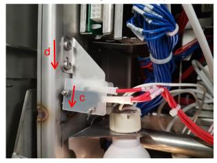
7 Adjust the bracket downwards (d) until the arm of the micro switch touches the housing of the micro switch.
