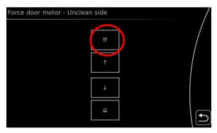
5 Ensure that the door is fully closed, and that the pulley is touching the bumper plate welded into the track for the door- if it isn't you must re-open the door and close it again:
