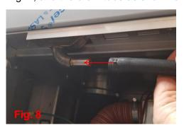
Locate the mains supply cable, mount the lead in bushing in the top plate and lead the cable through.
