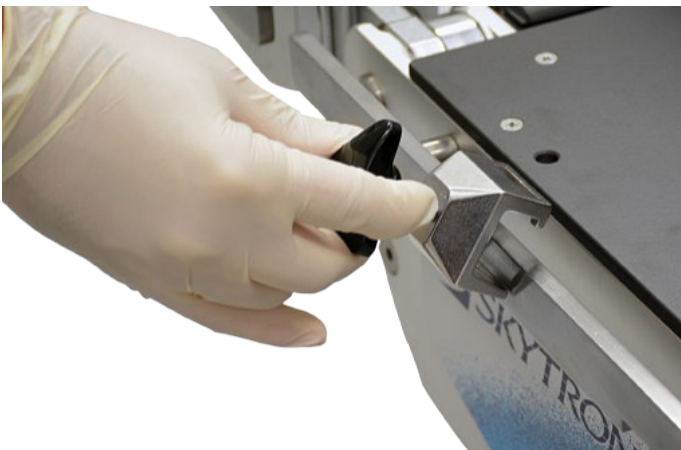
Figure 1. Install the Bar Clamp
